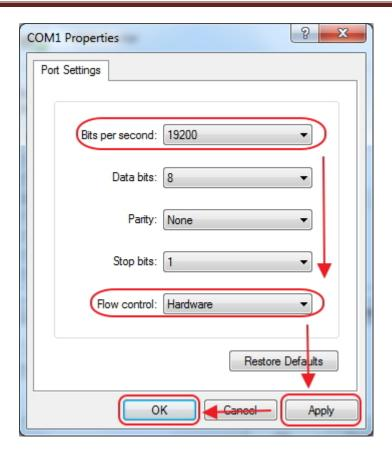
"Bit per second" means Serial port baud rate, it must same as printer setting. For example, if printer baud rate is "19200bsp", then you must select "19200" on "Bit per second", just as above picture. (Factory default baud rate is 9200bps)
